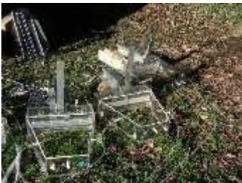
Figure 1 Chamber system for (CO 2 ) soil measurements
